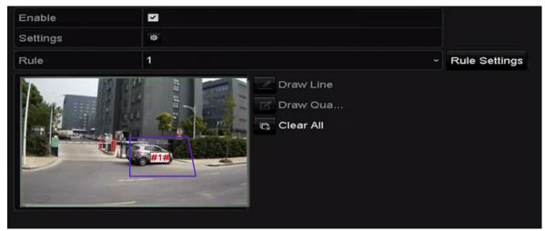
Figure 9-6 Draw Area for Intrusion Detection
