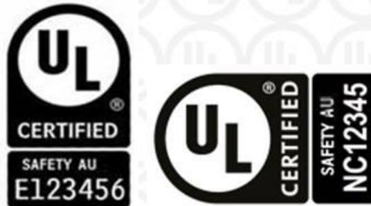
The UL Enhanced Mark may appear on a label, nameplate, or may be cast, stamped or moulded into the product. When appearing on a label or nameplate, the Manufacturer's name or trademark along with a model number are also required on that same label or nameplate. If cast, stamped or moulded, the Manufacturer's name or trademark and model number shall also appear elsewhere on the product.
