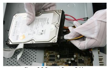
Figure 2-3 Connect Power Cable
