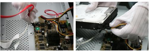
Figure 2-2 Connect Data Cable
